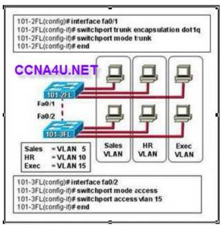
Configure port Fa0/2 on switch 101-3FL as a static trunk link
