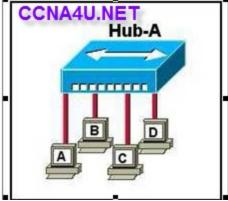
The hosts transmit a jam signal to ensure that all hosts on the network are aware that a collision has occured
